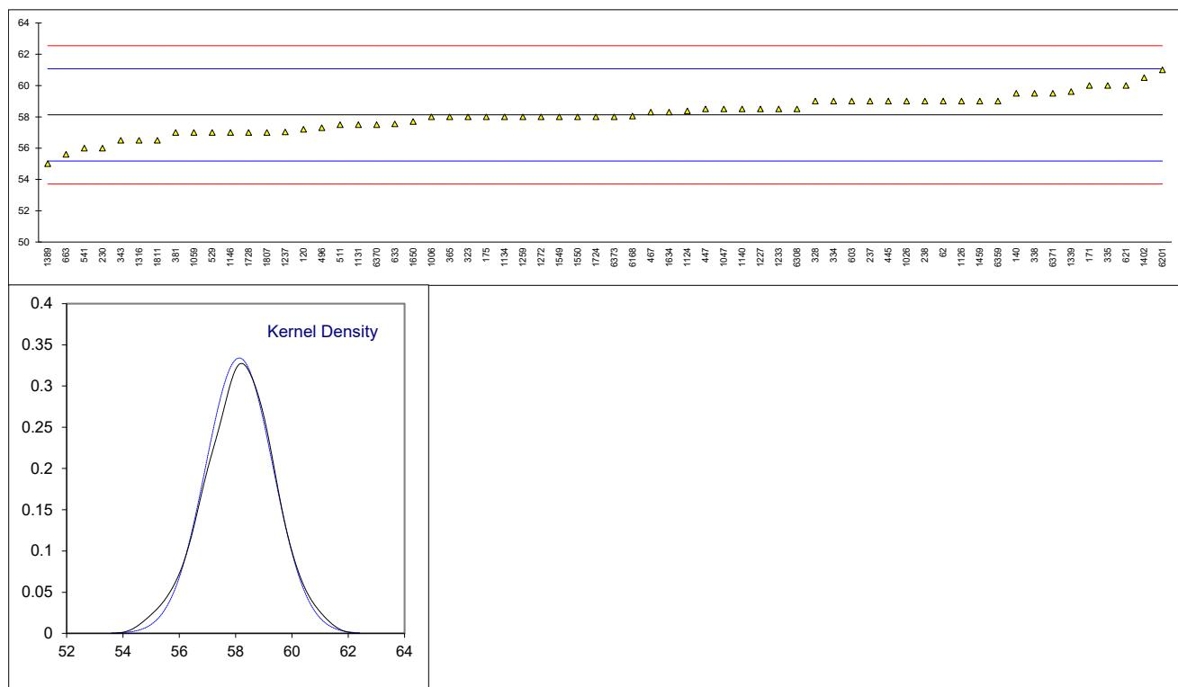
Determination of Kinematic Viscosity at 40°C on sample #21070; result in mm<sup>2</sup>/s
